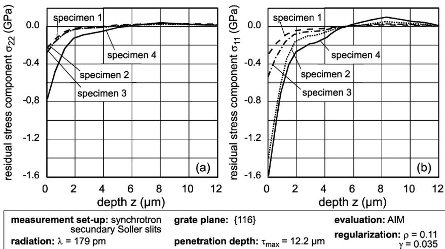
Fig. 3. Calculated residual stress depth profiles depending on the depth  $z$  for the stress components  $\sigma_{11}$  (b) and  $\sigma_{22}$  (a) corresponding to the data from Fig. 2. The regularization parameters of the AIM [see Eq. (10)] are chosen as indicated in the box above.
