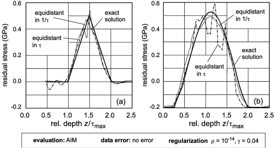
Fig. 1. Achievable accuracy, reconstructions with synthetic data,  $\tau_{max}$  denotes the maximal penetration depth corresponding to the reflection angle  $\theta_0$ . Curves of a continuous function (a) and a continuously differentiable function (b) have been used.
