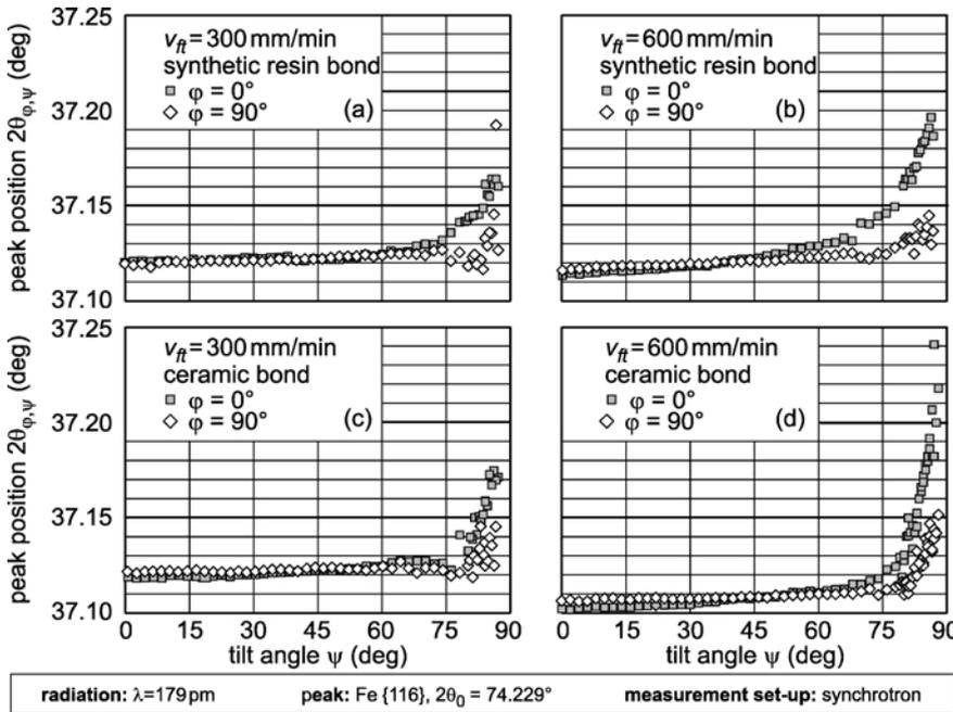
Fig. 2. Measured peak positions using low (a, c) and high feed rates (b, d). The bond types have been varied: (a, b): synthetic resin bond, (c, d): ceramic bond. The peak positions were measured using two rotation angles  $\phi = 0^\circ$  and  $\phi = 90^\circ$ .  $\lambda$  denotes the wavelength.
